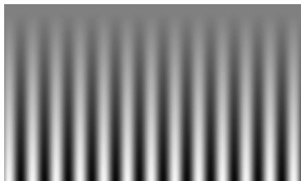
Fig. 3. Example of sinusoidal grating stimulus. Along the vertical axis of the screen, contrast becomes the highest in the bottom and lowest in the top of the pattern.
